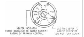
Fig. 4 - Adjustable Heater
